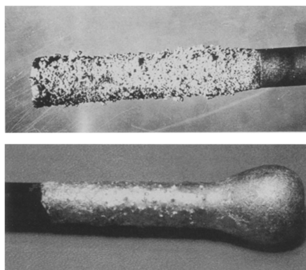
Fig. 4. Titanium diboride coated carbon rod (EK 78, Ringsdorf) (a) before and (b) after 500h of cathodic aluminium deposition. The coated parts of the electrode are completely wetted by the aluminium whereas on the exposed carbon rod no aluminium is deposited as Al-deposition on carbon occurs at a sizeable cathodic overpotential.
